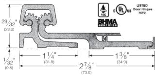
CFS83 - Full surface units are designed primarily for retrofit work and are applied to the exposed surface of the door & frame
