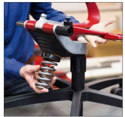
Trimension® with direct control and central spring: the two swivel arms are part of the mechanism and (depending on the movement direction) press the springs together or move them to the sides.
