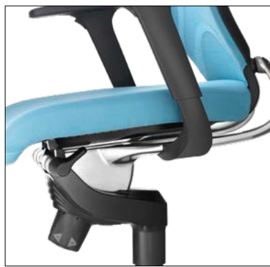
Trimension® with direct control and central spring: the two swivel arms are part of the mechanism and (depending on the movement direction) press the springs together or move them to the sides.
