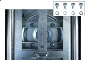
Locate four  $1/4" \times 1/2"$  bolts and four spring washers in parts bag. Tighten screws with washers firmly into four holes.
