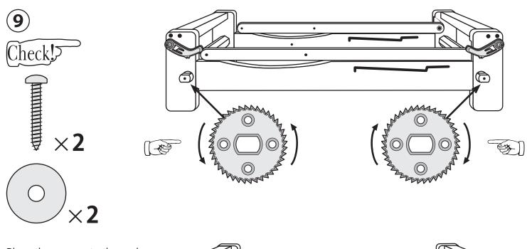
Place the cogs onto the ends of the rollers. Check the teeth engage the pawl. THEN secure with washers with small holes and 20mm (3/4") screws.
