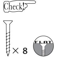
Assemble the castle with 8 screws. Check! Only use 30mm  $(1^{1}/4^{"})$  screws. Longer screws may damage the castle side.
