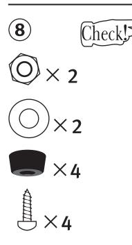
Attach the 4 rubber feet with the 12mm ( $\frac{1}{2}$ ") screws. Attach the support arms to the loom sides after checking they are the correct way around. Secure with washers and nuts. Leave 0.5mm (1/32") gap under the head of the washer and nut.
