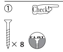
Assemble the castle with 8 screws. Check! Only use 30mm  $(1\frac{1}{4}")$  screws. Longer screws may damage the castle side.
