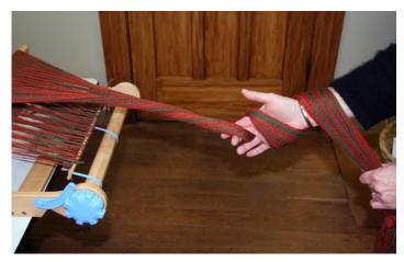
4. Stand at the back of the loom and twist the threads as shown, ensuring you keep the same firm tension.
