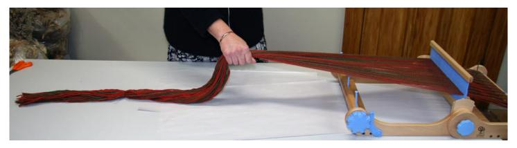
1. Start warping the loom as per the instructions until you are ready to cut the threads at the warping peg. Cut the threads at the warping peg. Hold the threads firmly approx 30cm (12ins) from the tie.
