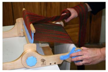
6. Insert a sheet of paper and continue to wind on the warp.
