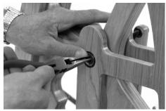
9. Replace the screws holding the back frame to the base and dowel spacers.10. Thread the flyer into the shaft.
