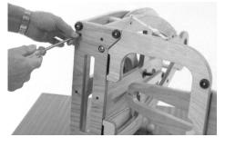
**4.** Use a hammer and nail to tap the flyer shaft and crank forward until they are free of the bearings in the back frame.
