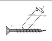
To make assembly easier use candle wax on the screws.
