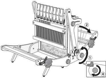
**Step 4:** Loosen knobs securing the beater supports, slide the beater completely forward and tighten the knobs.
