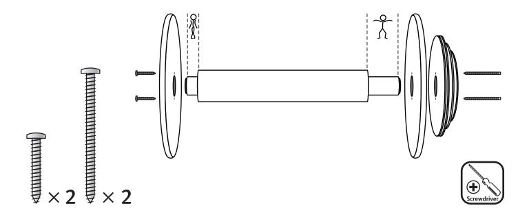
Assemble the bobbin by aligning the screw holes in the bobbin end, whorl and long end of the bobbin centre. Then push the bobbin end and whorl onto the bobbin centre keeping the holes aligned and secure with 50mm (2") round head screws. Align the screw holes in the other bobbin end and short end of the bobbin centre. Push the bobbin end onto the bobbin centre keeping the holes aligned and secure with 25mm (1") round head screws.
