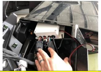
Hold off on connecting the power until the kit is completely installed and everything is wired and attached.
