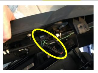
Step 6. Run the long wires from the front to back of the machine:
