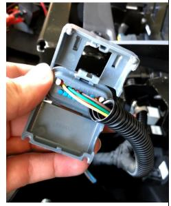
6. Insert pins into plug and make sure they line up evenly with the other existing pins. The **Black** wire will go in position **6**, and the **Red** wire will go in position **7**.
