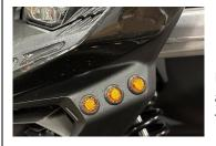
Install the rubber grommet into each hole from the front making sure they are seated fully. Next, push the amber LED into each grommet from the front to secure.
