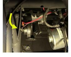
Locate the harness on the back side. Route the black and red spade connectors to the horn and connect them to the two flat terminals on the housing. These spade connectors are reversable and can be connected in either direction.
