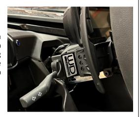
Next, run the wire on the column switch with the "white" 4-pin connector following the factory wiring for the instrument cluster under the dash. We will connect it to the control module in a later step.
