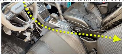
Follow the Factory Harness behind and up the rear firewall (Green Line, Below), then under the driver's rear fender all the way to the driver's side taillight (Yellow Line, Below). Make sure to secure this cable away from any hot or moving components.
