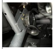
Make sure that no moving parts can contact the horn when mounted. We recommend mounting on the left frame under the dash on the driver's side (Shown, Left). If you do not want the horn in the cab, you may also mount it to a bolt on the outside of the firewall (make sure it does not contact the suspension when it is compressed.
