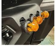
Starting on the driver's side, locate the side of the harness with the driver's side label on the wire close to the LEDs. Slide the rubber grommets off the three LEDs down onto the black and white wires. Next, slide each of the amber LEDs though the **back** side of holes you drilled, followed by the rubber grommets (Shown, Left).
