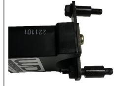
Next, Locate the two, long, partially threaded bolts and plastic spacers in the bag of mounting hardware. Insert one bolt through each hole on the pre-attached bracket on the turn signal switch. Install one spacer over the threaded end of each bolt on the other side (Shown, Left).
