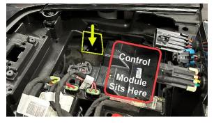
Once the control module has been positioned, feed the extension wire for the column turn signal switch (covered in black wire loom with a 4-pin "white" connector) under the dash using the space shown (Yellow Highlights, Left).
