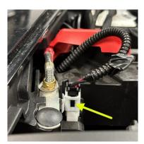
If this connector is used by other accessories on your machine, you can connect the power and ground wires on the control module to the screw posts directly behind the accessory connector location.
