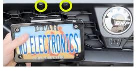
Before mounting the bracket, feed the 2-pin connector on the power extension cable through a hole in the rear grill and route it to the driver's side taillight adapter.
