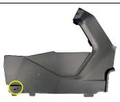
The first panel is in the drivers footwell on the right side. The panel is held in by one plastic clip on the very front bottom corner of the panel, below the gas pedal (Yellow Circle, Left). Once this clip is removed, the panel is held in with clips on the rear and can simply be pulled towards you to release the clips and remove the panel.
