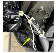
Start on the passenger's side. Connect the 3-pin WD taillight adapter with the long white wire into the passenger's taillight housing and connect the factory harness to the other end of the WD adapter. Feed the white wire with the female bullet connector behind the rear bumper across to the driver's side taillight following the factory harness as closely as possible (Yellow Arrow, Left).
