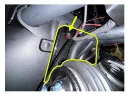
Now, route the passenger's side of the harness, following factory wiring as closely as possible, to the holes you drilled on the front passenger's corner, and repeat the installation steps you used on the driver's side. Once the LEDs have been installed. Run the 4-pin connector, up through the grommet in the firewall next to the factory harness, up to the control module, and connect it to the mating connector (far left when facing the WD Logo).
