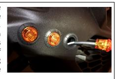
7b. Installing the Front Turn Signals (Sequential LEDs)
