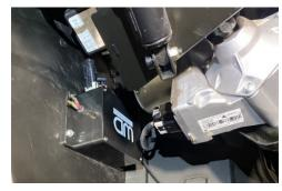
3. Attach the column-mounted turn signal lever
