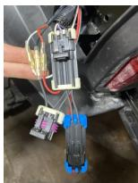
The bullet connectors on BOTH taillight adapters will match up to the same colors that are on the long black cable you ran in step 5. Red to red, white to white, and black to black. There are only three total wires with bullet connectors between the two adapters. The Red and black wires are on the driver's side adapter (the one with the blue 2-pin connector) and the white wire is coming from the adapter you ran from the passenger's side taillight.
