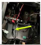
side down the hole in the center console that routes into the center tunnel. Then run the length of the cable all the way back to the driver's side taillight.
