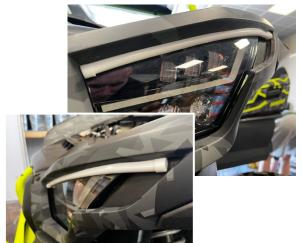
Zip tie the <u>LED Drivers/Ballasts</u> under the Hood, and connect them to the Sequential LEDs being very CAUTIOUS routing the wires around any hot surfaces. Zip tie them out of the way. Connect the LED Drivers to the end of the Sequential LED strip then run the other side to the Main Control Module.
