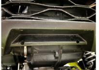
Run the power wire up under the driver's side fender and find the factory accessory plugs there. Connect the Red to the Power wire (red) and the Black to the Negative wire (black with yellow stripe). (if your plate doesn't illuminate when you turn the key on, simply flip these wires.)
