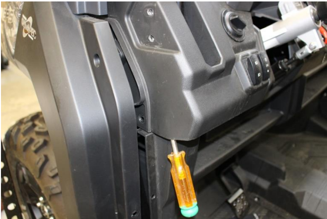
PRY DASH OUTWARDS WHILE DRILLING PILOT HOLE
