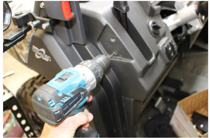
DRILL A 1/8" PILOT HOLE IN PREMARKED PLASTIC
