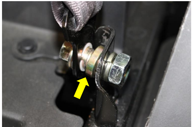
Remove bolt and discard this 1/8" washer
