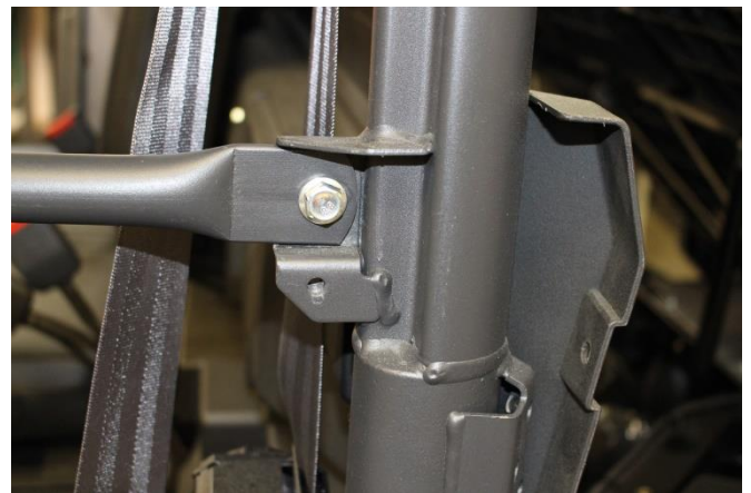
Exposed shoulder bar mount
