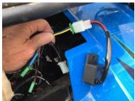
**Self-Canceling Flasher Relay Feature**: The SELF-CANCELING FLASHER RELAY has a timing circuit that will cancel the turn signals after three minutes and thirty three seconds. The timer is reset whenever the turn signal switch is returned to the center/off position.
