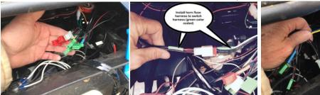
5. Secure the switch harness to a cross member using a cable tie. The flasher relay and can be bundled and secured with a cables tie to the switch harness.
