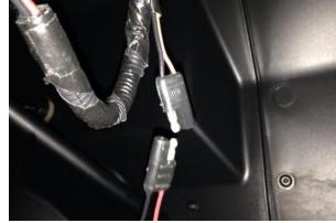
SAE adapter is located in front of the firewall, under the front hood.
