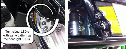
16. Connect the front turn signal harness to the 4 pin connector on the switch harness with the RED sleeve match marking.
