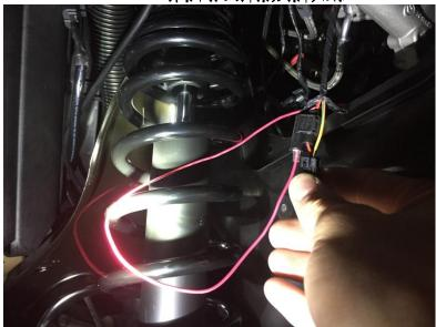
NOTE: Check orientation of parallel tap to insure access for the male connector prior to seating the parallel tap connector with pliers. You can unplug the connector to allow easier access.
