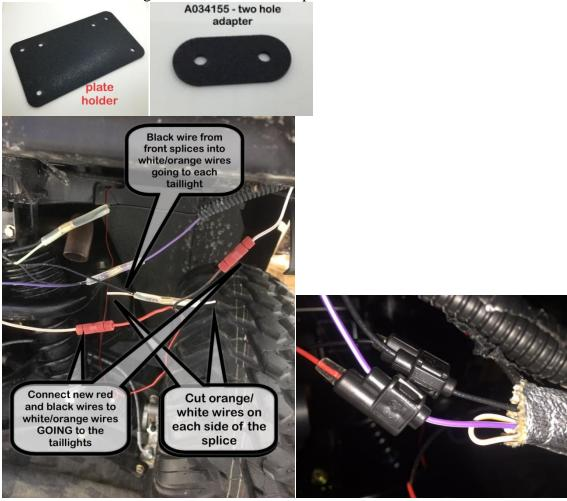
NOTE: Check orientation of parallel tap connectors to insure access for the male connectors prior to seating the terminal with pliers.
