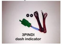
The dash mounted turn signal indicators interface is a 3 pin connector with **blue** color coding.
