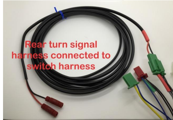
The horn, power (fuse holder) and ground wires interface is a 4 pin connector with green color coding.
