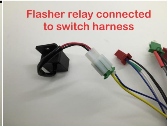
The flasher relay interface is the only 3 pin connector with no color coding.
