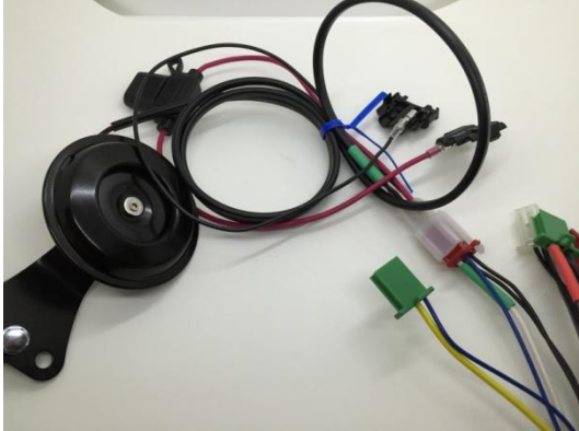
The horn, power (fuse holder) and ground wires interface is a 4 pin connector with green color coding.
