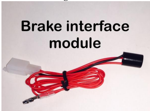
The brake light interface module harness is the only 2 pin connector and has no color coding.
