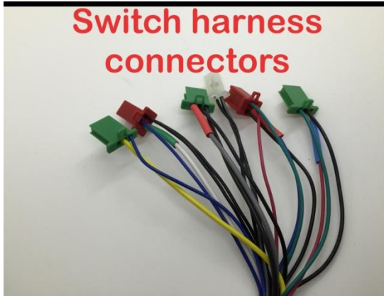
The flasher relay interface is the only 3 pin connector with no color coding.
