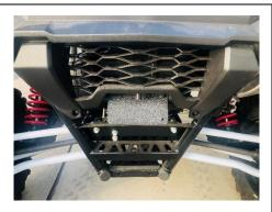
**EXPLANATION**: The LICENSE PLATE LIGHT is installed in the single hole where the light will shine on the license plate.
