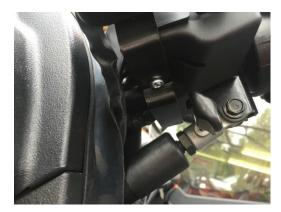
**NOTE:** You may need to put some pressure on the SWITCH BRACKET to force it over the tilt mechanism bracket, and again to align the hole with the provided SPACER and fastener. You may also need to squeeze the bracket once it is place to get the nut started.
