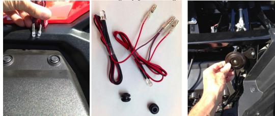
NOTE: Where possible run new cables adjacent existing wires, utilize existing cable anchors where practical. Insure wiring does not contact moving or hot components.
