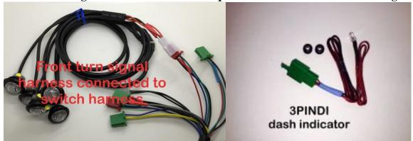
The front turn signal harness interface is a 4 pin connector with **red** color coding. The dash mounted turn signal indicators interface is a 3 pin connector with **blue** color coding.
