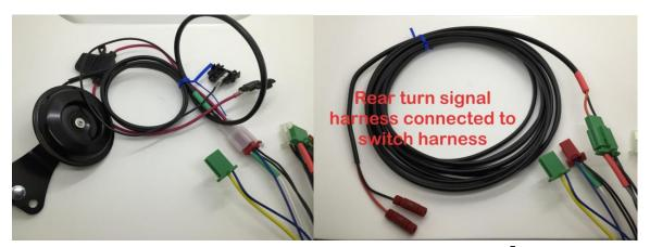
The rear turn signal harness interface is a 3 pin connector with red color coding.
