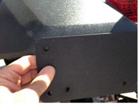
28. Install the license plate holder by drilling mounting holes in either to the rear plastic or the rear support member.
