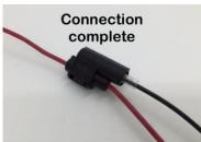
29. Locate the brown (12 V DC, taillight) and green (ground) wires leading to the rear taillight assembly and install a parallel tap connector on each wire and connect the red wire from the plate LED to the brown wire and LED black wire to the vehicle green wire.
