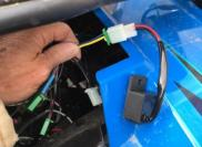
7. Secure the switch harness to a cross member using a cable tie. The flasher relay and can be bundled and secured with a cables tie to the switch harness.
