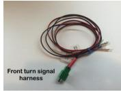
11. Install the front turn signal wiring harness to the switch harness 4 pin connector with red color coding.
