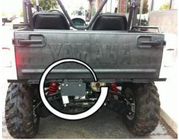
25. The plate light can be installed as one of the four license plate bolts or can be installed in the two hole adapter where the light will shine on the license plate. The plate light/2 hole adapter is secured to the license plate holder using one of the four license plate bolts.
