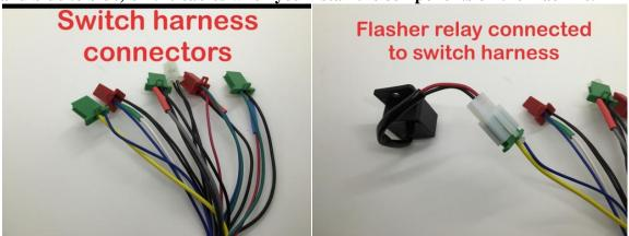
The flasher relay interface is the only 3 pin connector with no color coding.
