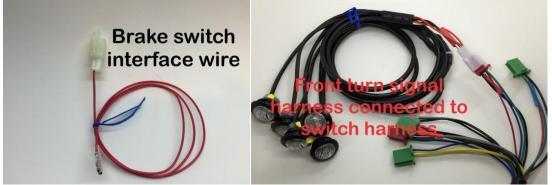
The brake light module is the only 2 pin connector and has no color coding.
