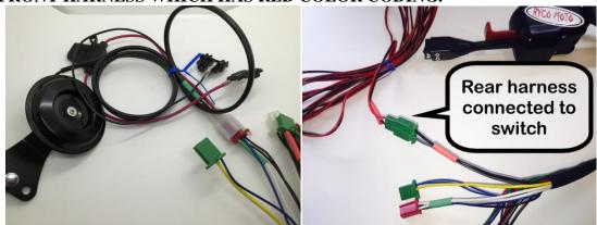
The rear turn signal harness interface is a 3 pin connector with red color coding.
