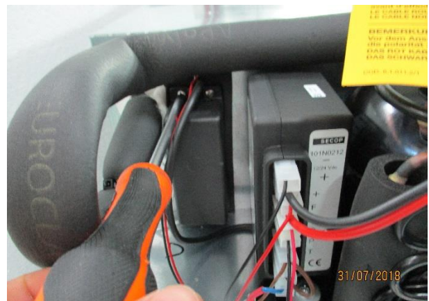
6. Remove the thermostat's box (3 bolts)
