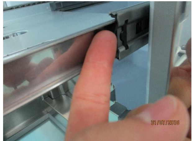
2. While you hold the hooks in reverse position, pull the drawer to remove it
