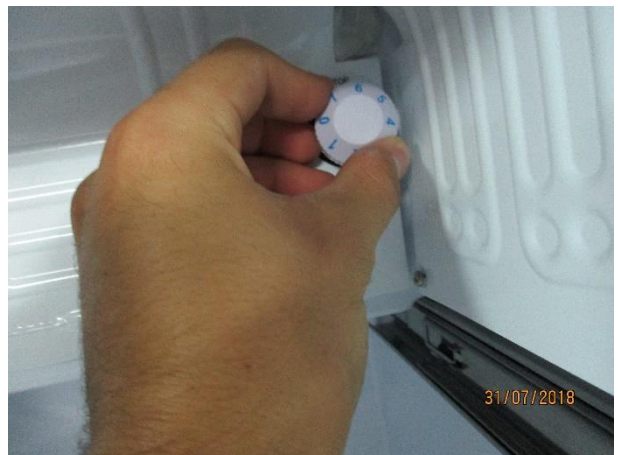
4. Remove the thermostat's knob
