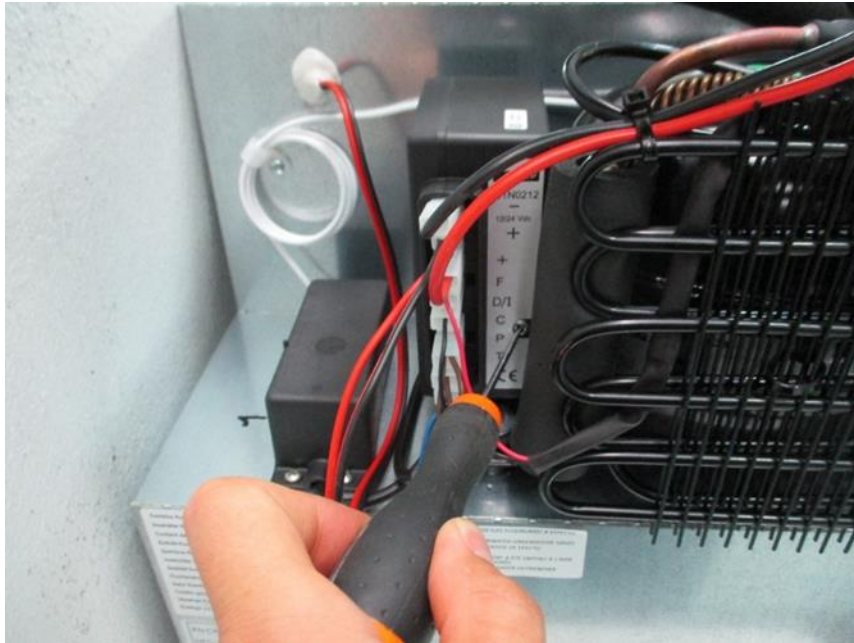
Unscrew the bolt fixing the ECU, and move the ECU
