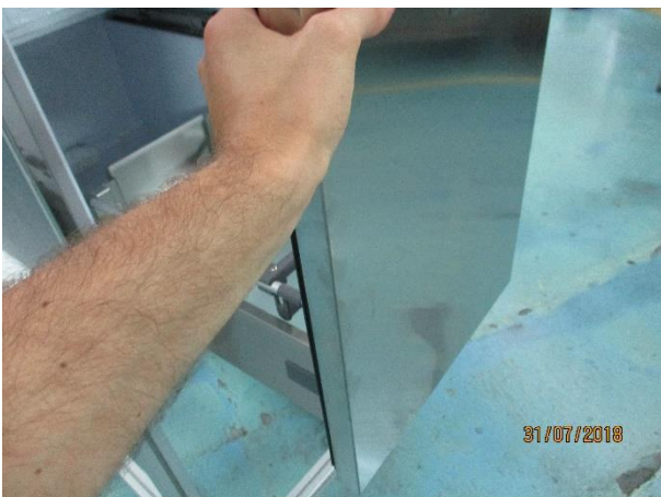
3. Pull up the drawer door and pull it out to remove it
