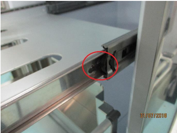
1. Switch the position of the hooks in both sides of the drawer (see the following picture)
