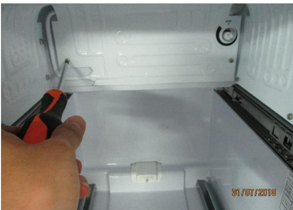
5. Unscrew the evaporator (7 bolts) to remove the thermostat bulb
