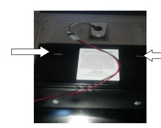
If your cabinet does not have a top mount bracket, use small black TF top bracket with black push clips and secure to bracket in the top of cabinet. This will bolt to TF top fridge bracket. If your truck already has top mounting bracket as shown here, the TF top bracket and push clips will not be needed.
