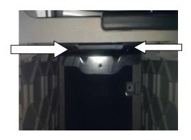
Slide fridge on to mounting plate, aligning rear finger tabs to fridge bottom plate. Insure wires are not pinched or rubbing.
