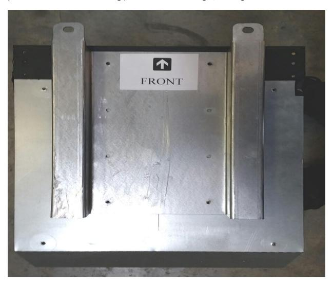
Turn fridge right side up and center top bracket 1/2" from front of fridge cabinet, centered side to side. (If silicone caulking available, apply a small amount to each screw hole in bracket to minimize potential of screws loosening.) Install bracket using 3/4" long #10 sheet metal screws. It may be necessary to predrill the 2 front holes due to the steel latch plate on the fridge.
