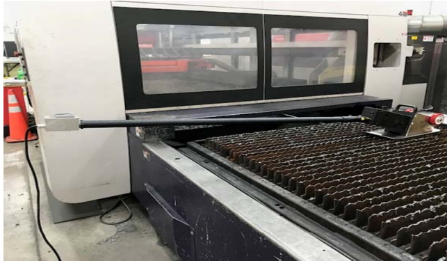
With switches off plug tool into a 220Volt outlet with a minimum of 5 Amp capacity
