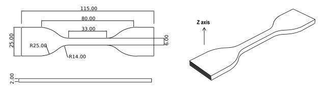
Tensile testing specimen; ASTM D638 (ISO 527, GB/T 1040)
