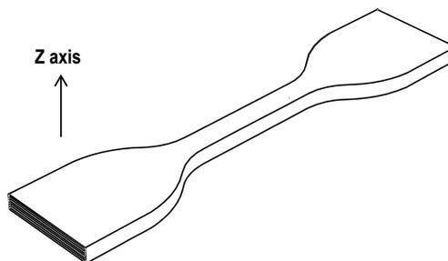
**Tensile testing specimen;     ASTM D638 (ISO 527, GB/T 1040)**
