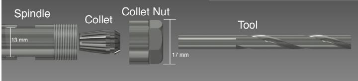
C). Place a 13 mm wrench onto the spindle's spanner slot. Due to the spindle's low torque, holding the wrench in place prevents spinning if accidentally enabled.
