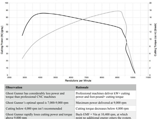
Spindle Cutting Power and Torque
