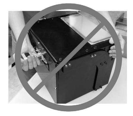
Place Ghost Gunner on a smooth surface in a shop environment conducive to stray aluminum chips. Ghost Gunner must operate in the upright position to prevent chip ingress to sensitive linear components.
