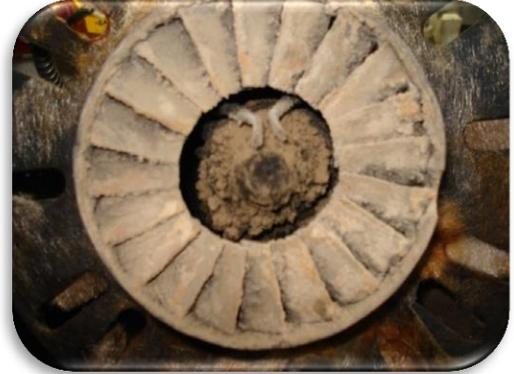
If you have a combustion analyzer it makes adjusting the burner settings very easy. For perfect combustion we expect these readings on your analyzer: CO<sub>2</sub> – 12%, O<sub>2</sub> – 6%, CO – less than 50 ppm, excess air – 30%, chimney temperature (in clean condition) – 350°F, smoke patch results of 0 to 2.
