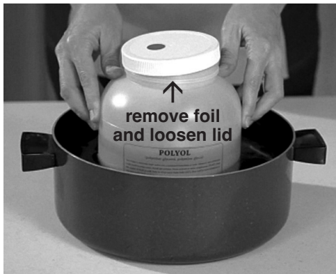
Remove the foil safety seal and loosen the lid of the container when heating the Polyol or Iso.
