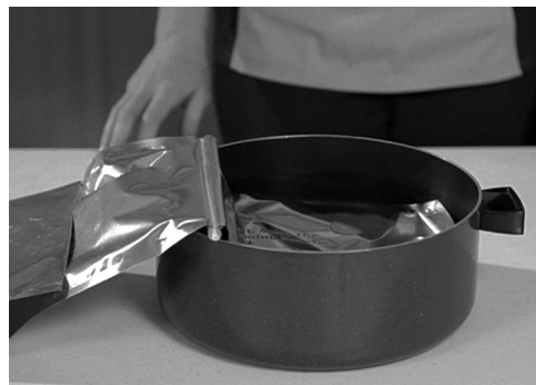
Place the Iso or Polyol section of the Bag Pack in a hot water bath to melt any crystals.
