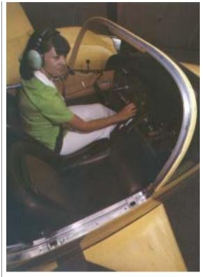
Seats in the cockpit of the Wing Derringer twinengine lightplane have temper foam padding to reduce pilot and passenger fatigue on long flights.
