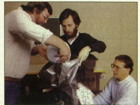
Foam-In-Place Seating is produced by mixing Sun-Mate ingredients, pouring the mixture into a plastic bag — which is later used as a mold — and contouring the mold to the most therapeutic body position. The seat is then upholstered and ready for use.
