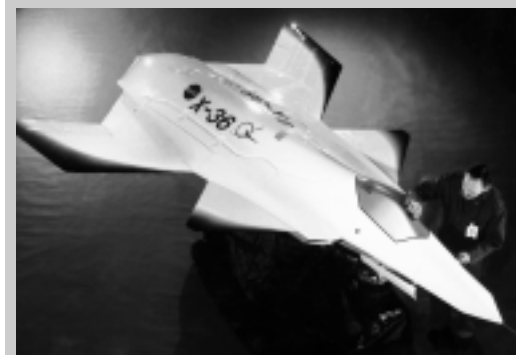
Subscale prototype (28%) of the model NASA/Boeing X-36 Tailless Fighter Agility Research Aircraft
