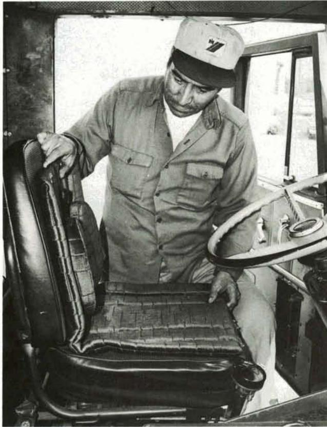
constructed of molded fiber glass and padded with Temper Foam to reduce pilot and passenger fatigue on long flights.
