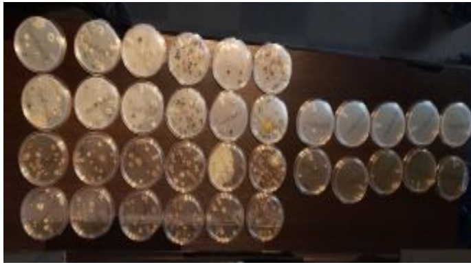
To insure accuracy, 40 tests were conducted on microbial resistance of lime coating in sealed plaster and paint boxes.
