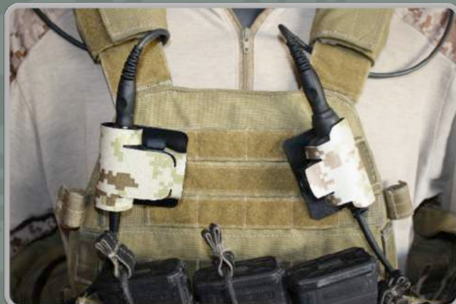
PTT Clamp – Nexus PTT on the left and TEA PTT on the right
