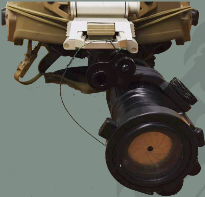
Tarsier Eclipse mounted on PVS-14 – with 25lbs lanyard
