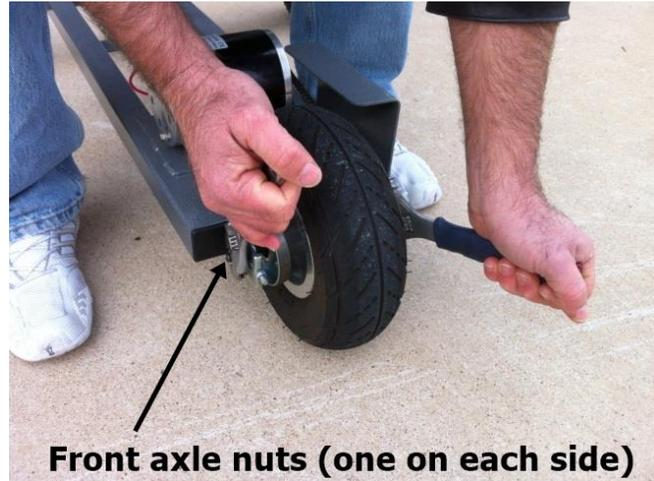
**Front axle nuts (one on each side)**
