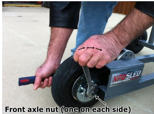
5. By moving both chain tensioners equally, the alignment of the front wheel should be preserved. Check alignment and if the XPO Trainer does not roll straight, follow the steps for alignment.
