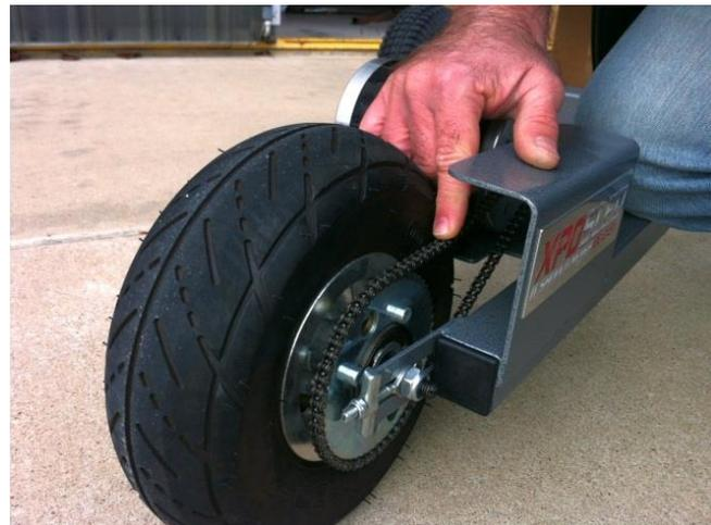
4. Place a wrench on both front axle nuts, and tighten by turning clockwise. It is best to tighten by pushing the wrench towards the rear of the XPO Trainer. Pulling the wrench towards the front of the XPO Trainer may pull that side of the axle forwards and ruin the alignment. It is not necessary to tighten forcefully.
