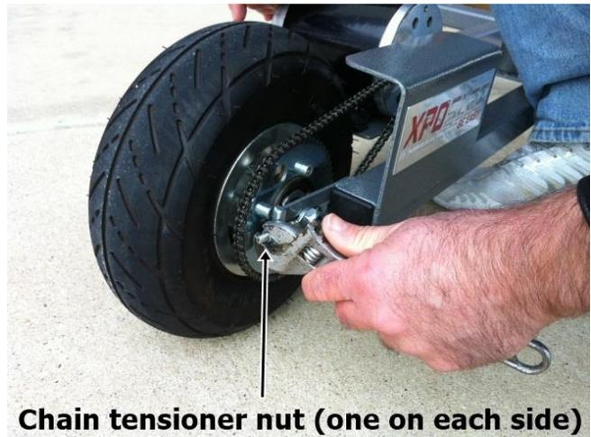
5. Repeat steps 3 and 4 until the XPO Trainer rolls straight. Be certain to check chain tension after every adjustment to avoid damaging the resistance motor. If at any point the chain is too tight, adjust BOTH chain tensioner nuts counter clockwise until the chain has loosened to  $\frac{1}{8}$ " flex under firm fingertip pressure and resume alignment.
