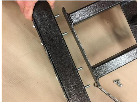
4. Using two 1/2 inch wrenches, tighten the nuts down firmly.
