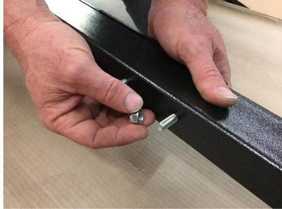
3. With the sawtooth kickplate oriented on the top side of the rear wheel assembly, align the holes in the front wheel assembly and slide the bolts through.
