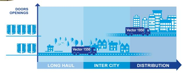
The unit selection may vary according to the type of goods transported, insulation of the box, size of the body, ambiant temperature, etc...
