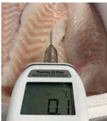
The temperature of the raw material is + 0,1°C before packaging.
