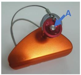
Unless the safety release button is first pressed, the pin should not be able to be removed.
