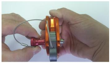
If, using reasonable force and without the safety button being pressed, the pin can be removed from the body of the THRG2 Rope Grab, please make a note of the batch number and:
