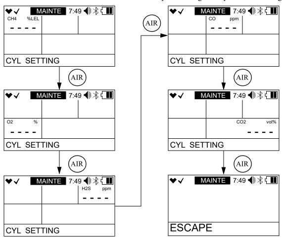
8. Press and release POWER MODE. The current setting will flash. In the example below, the combustible gas channel is selected.
