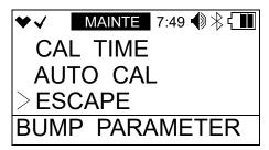
2. Press and release POWER MODE. The instrument will return to the **BUMP PARAMETER** menu.
