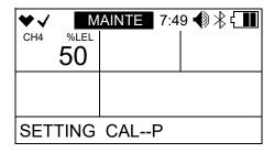
9. Use AIR to adjust the calibration gas value. The calibration gas value in the instrument must match the value listed on the calibration gas cylinder you are using for that channel.
