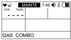
3. Press AIR to scroll through to the instrument channel whose target gas you want to change.
