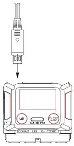
Figure 8: Connecting the Charging Cable
