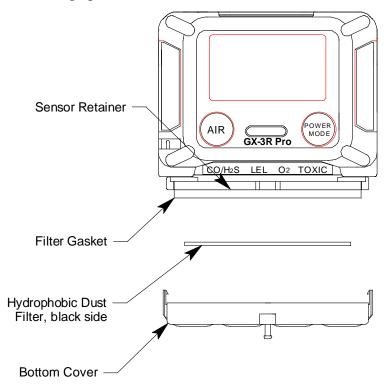
Figure 11: Replacing the Hydrophobic Dust Filter
