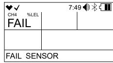
Press and release POWER MODE to acknowledge the failure and continue. The gas reading for the failed sensor will be replaced by "- - - -". Replace the failed sensor as soon as possible.
