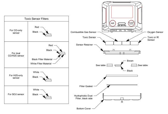
Figure 12: Replacing a Sensor
