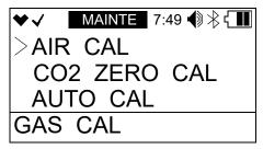
5. Press and release POWER MODE. The example below shows the standard 4 sensors (combustible gas, O<sub>2</sub>, CO, H<sub>2</sub>S).
