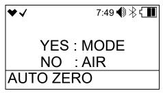
WARNING: Make sure that the instrument is in a known fresh air environment (an environment free of combustible or toxic gases and of normal oxygen content, 20.9%) before performing an auto zero operation. If you perform an auto zero operation in an area with gases present, the adjustment will not be accurate.
