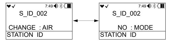
2. To change the Station ID, press and release AIR. The current Station ID will flash.
