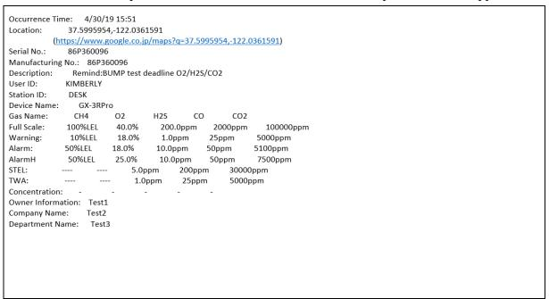
Figure 13: Email Alert for Past Due Bump Test
