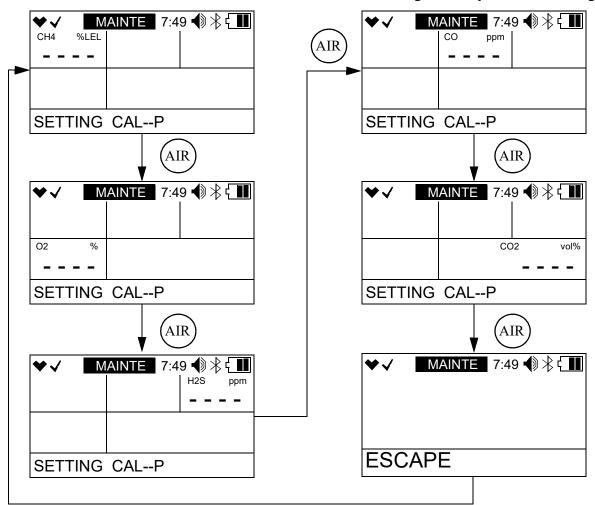
8. Press and release POWER MODE. The calibration gas value will begin to flash. In the example below, the combustible gas channel is selected.
