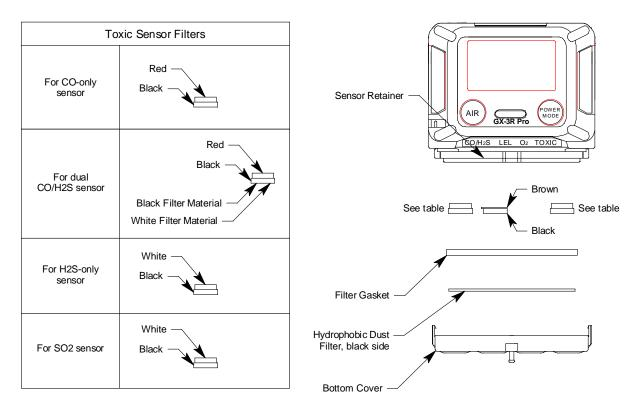
Figure 10: Replacing the Filters
