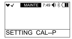
6. Press and release POWER MODE. The combustible gas channel will display.
