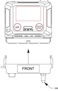
Figure 7: Calibration Cup Installation
