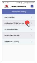
3. Turn the calibration and bump test reminder screens on or off with the toggle buttons. Set the calibration and bump test intervals.
