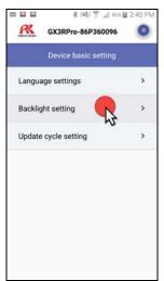
7. Set how long (in seconds) you want the backlight to stay on after each button press. The options are 0-255 seconds. The factory setting is 30 seconds.
