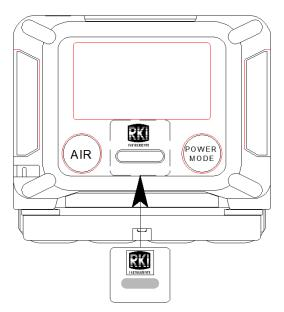
Figure 9: Buzzer Cover Replacement
