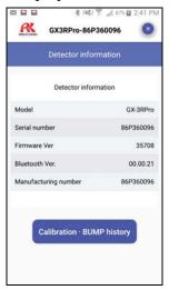
4. To view information for the last successful calibration and bump test, press the "Calibration BUMP history" button.
