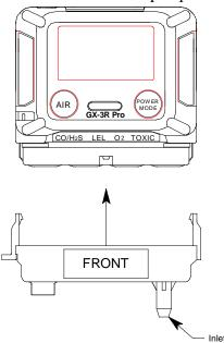
3. Use the tubing to connect the regulator to the inlet of the calibration cup.
