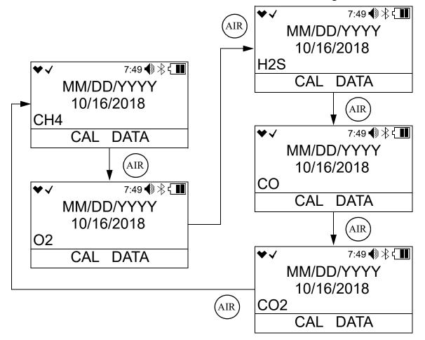
3. When you are done viewing the last calibration date for the sensors, press and release POWER MODE to return to the **CAL DATA** screen in Display Mode.
