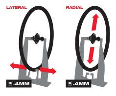
Lateral and Radial runout not to exceed 0.4mm縱和向橫向跳動不超過0.4mm°
