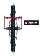
Wheel to be dished within 0.4mm (centerline of rim to centerline of hub) Unless otherwise specified by the frame manufacturer, rim to be dished to centerline of hub.輪組組 裝後, 縱向和橫向偏擺, 需低於 0.4 mm以內 (輪輞中心線到輪轂中心線)。
