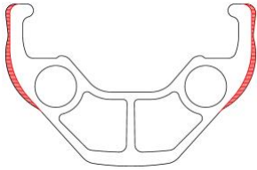
Drawing of Rim Profile Cross Section with Unbendium Bulge
