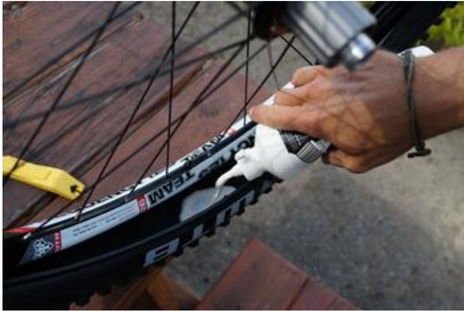
Pouring in WTB TCS sealant to unset portion of WTB TCS bead.
