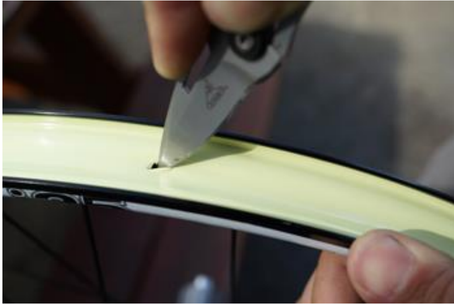
Carefully making valve cut with a small pocketknife.
