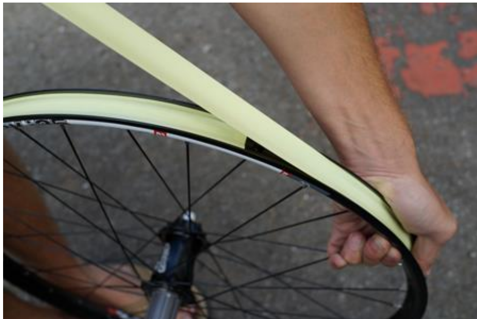
Approaching where the taping began, continue taping roughly 4 inches beyond the valve hole.
