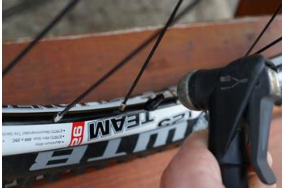
Attaching pump head directly to WTB TCS valve without core for faster inflation.
