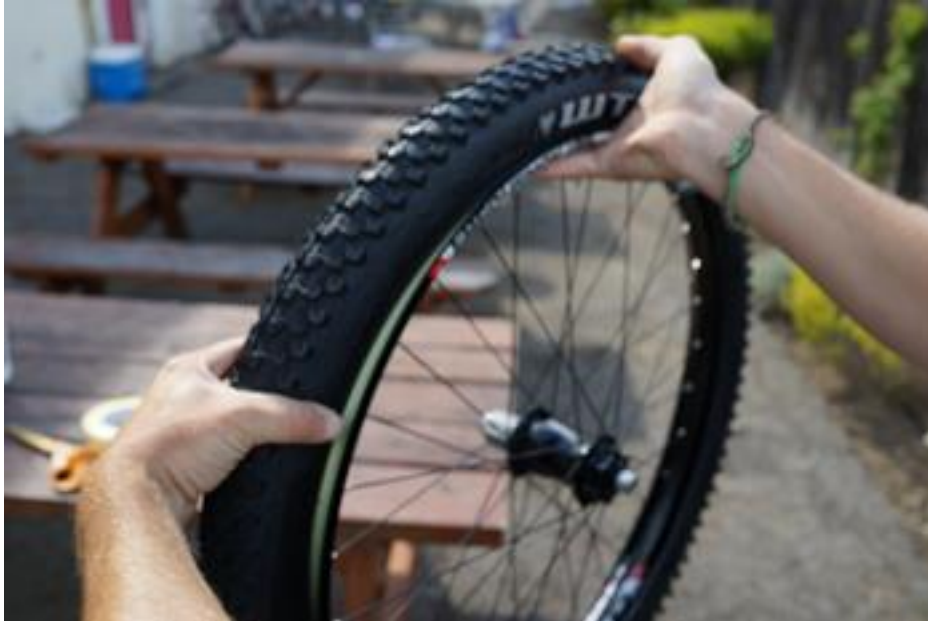
Continuing to set the bead with the left thumb while holding the tire on with the right hand.
