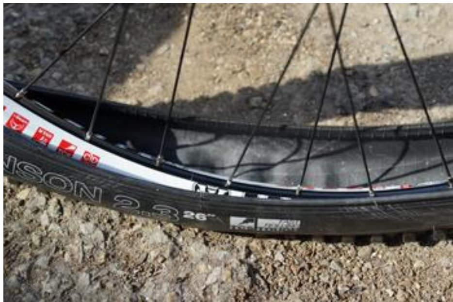
Placing WTB TCS rim within the U shape created by the WTB TCS tire.
