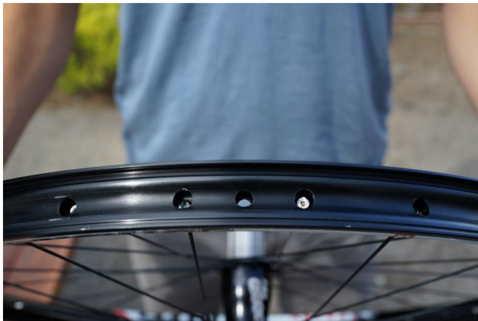
The valve hole in the WTB TCS rim is easily identified by closer spacing of three holes in the rim as seen above.
