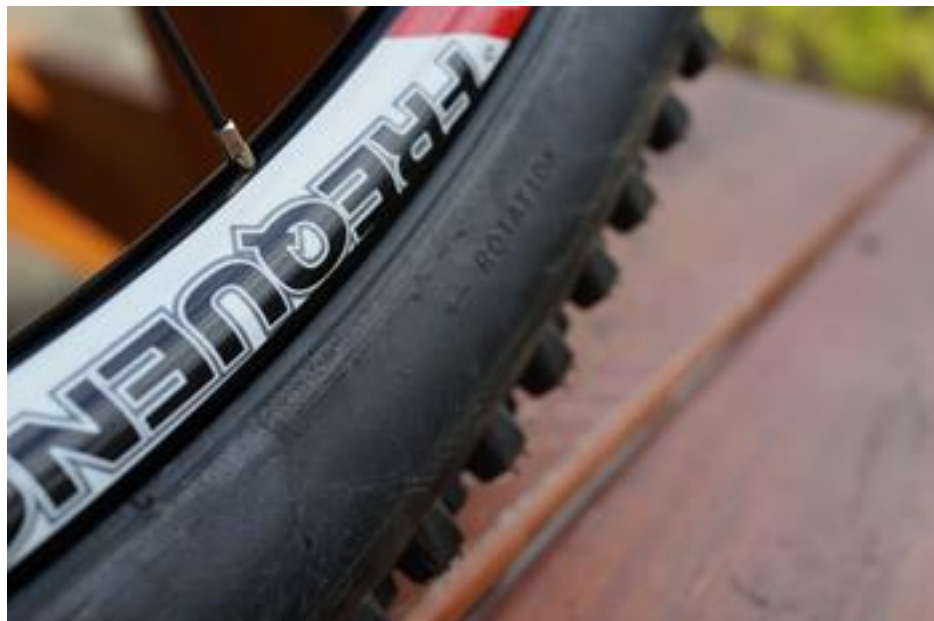
Chamfer tape line directly beneath rim and Frequency rim graphic. Also visible: Rotation indicator.
