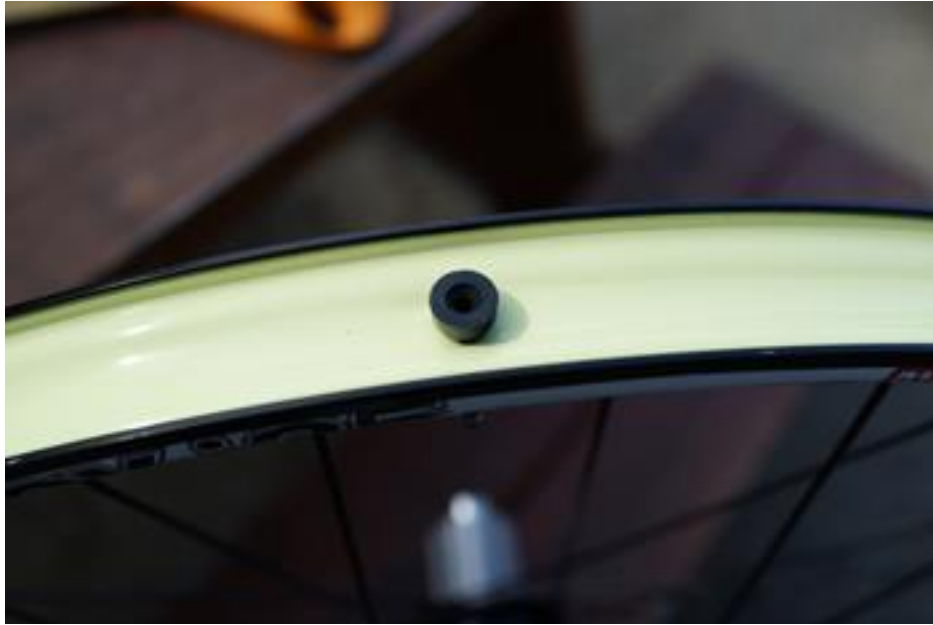
Conical plug of WTB TCS valve visible within WTB TCS rim's inner rim profile.
