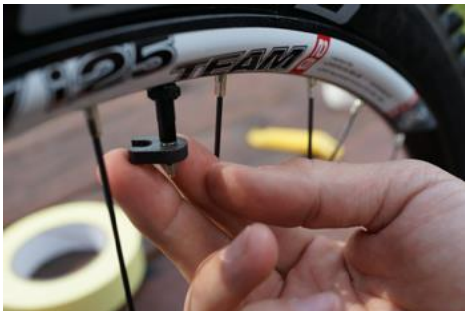
Using valve core remover to take out TCS valve core.
