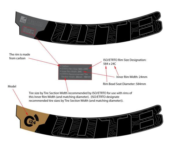
On the WTB Ci24 27.5" rim sticker shown above, the Rim Bead Seat Diameter is 584mm and the Inner Rim Width is 24mm, meaning this is a "27.5" / 650b" Mountain Bike Rim" with a 24mm Inner Rim Width and a 584mm Bead Seat Diameter. The Rim Size Designation is 584 x 24C.
