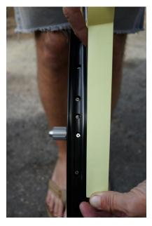
Start to apply WTB TCS tape roughly four inches before valve hole in WTB TCS rims.
