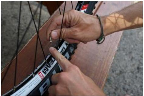
Rethreading the removable valve core into the WTB TCS valve. It can be a good idea to hold a finger over the open valve, as shown above, to prevent pressure loss.
