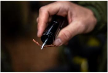
It's not necessary, but I like to fold back the plug's tails like this.
