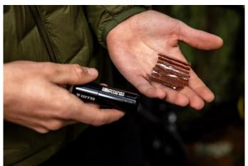
**Rocket Launcher**. This helps push the plug-loaded-anchors into the tire, and can be lengthened or shortened to suit your needs.
