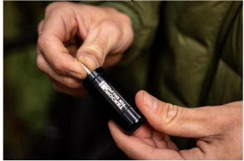
By optimizing the Launcher's length, you'll minimize the risk of pushing the anchor too far and damaging the tubeless tape.
