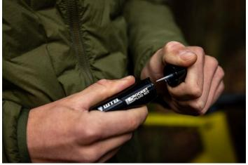
Push the pointy end into the puncture until you hear the leak stop. Rotating clockwise as you push can make that a little easier.
