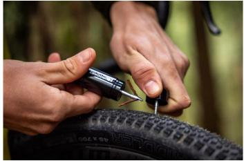
As before, rotating clockwise as you push will make it easier to push the Anchor through the hole.
