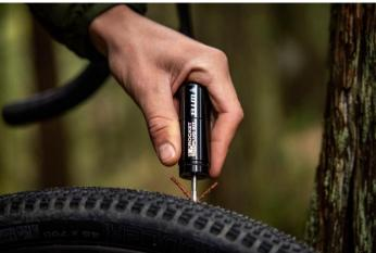
Once the Anchor has disappeared through the puncture and into the tire, pull the Rocket tool back out to leave only the tails of the plug visible.
