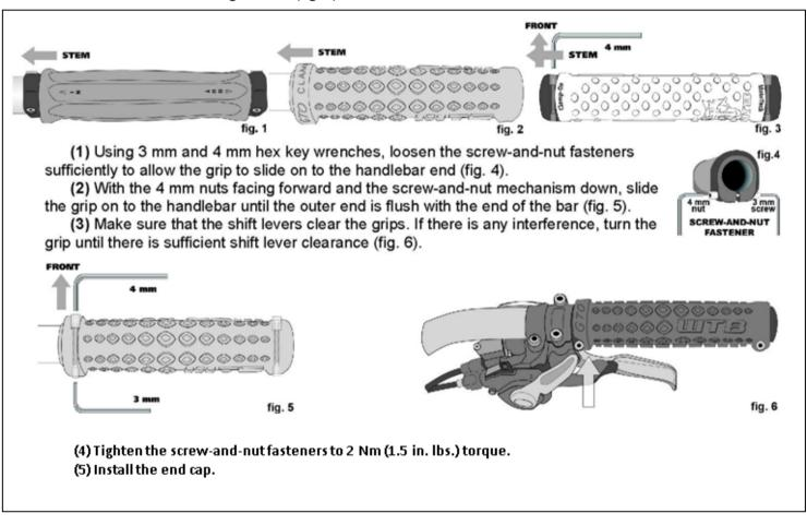
**d. To remove "Clamp-On" grips:** Remove the end cap. Using 3 mm and 4 mm hex key wrenches, loosen the screw-and-nut fasteners sufficiently to allow the grip to slide off the handlebar end.
