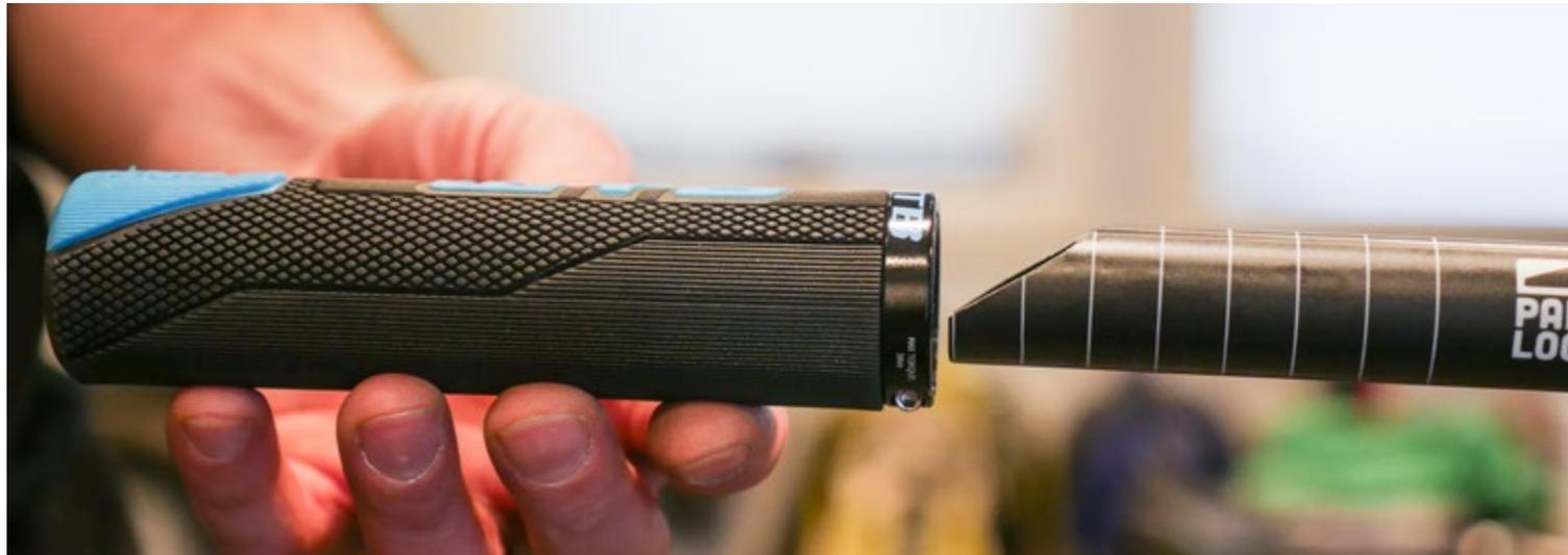
**11.** With the handlebar cut at the appropriate angle, slide the PadLoc grip onto the bar. Make sure the wedge is facing upwards.
